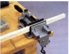
Although it has a relatively small holding capacity as a bench vise, it's ideal for gripping round stock or small objects that you're planning to drill on your drill press.
